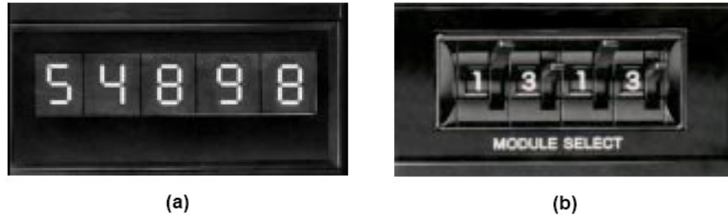
Figure 2-7. (a) A seven-segment indicator field device and (b) a thumbwheel switch.
